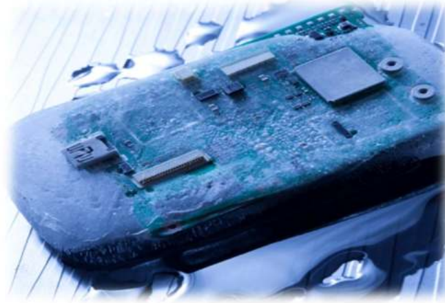
Figure 11: Representation of conformal coating protecting PWB with multiple components and solder joints. Besides having ability to prevent penetration to the PWB by moisture-water and harmful gases, the conformal coating must also withstand thermal cycling and thermal shock induced interfacial stress and stress concentration at corners and solder joints.
