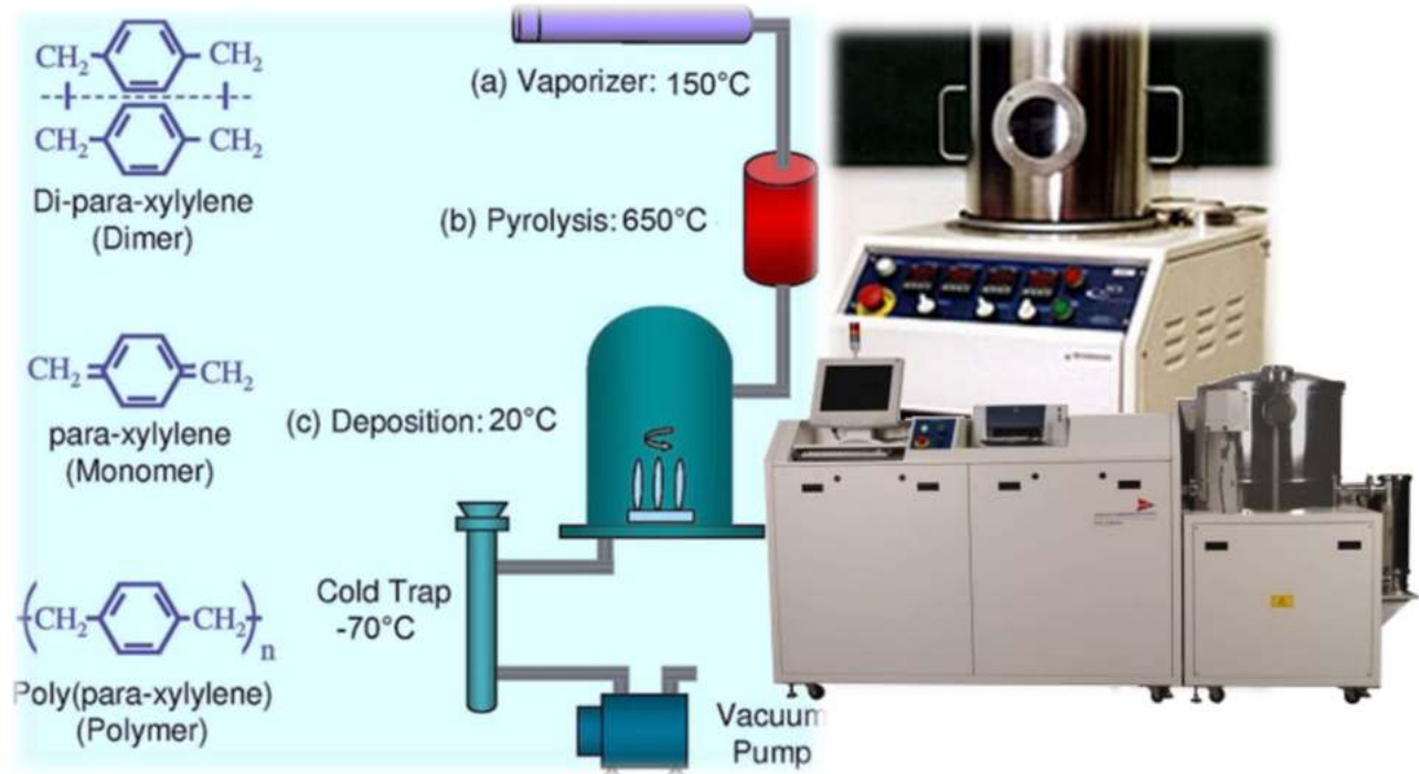
Figure 14: Parylene and the proposed ultra-thin oxide conformal coatings have to be deposited under stringent vacuum and temperature conditions. Not only raw material costs are substantially higher for Parylene, the application process cost and time are also limitations.
