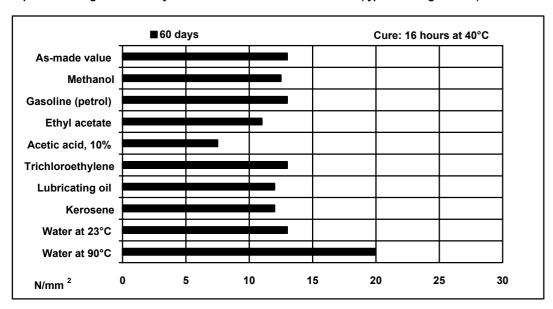
Lap shear strength versus tropical weathering (40/92, DIN 50015; typical average values)
