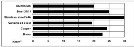
Cured for 24 hours at 23°C  $\,$  and tested at 23°C. Pretreatment - Sand blasting
